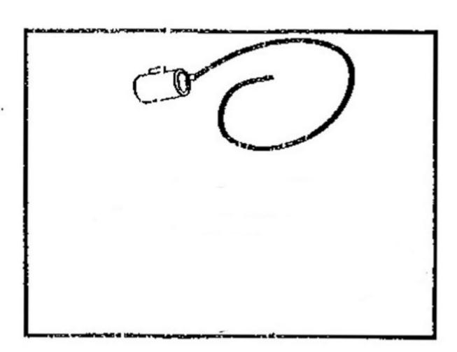
Select a straight portion of the cable and remove a section of the jacket measuring 24mm minimum to expose the outer copper braid or shielding being careful not to damage this.
