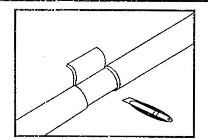
Remove the section of the sheath / outer jacket you have cut and clean the outer conductor / braid to ensure that a good connection will be made.
